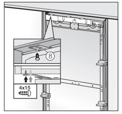
■ Screw the attachment plate lugs ® to the overhead furniture/fixtures.
